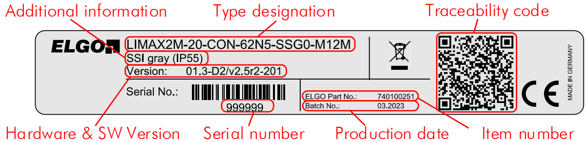
Fig. 1: Type label for identification of the sensor
